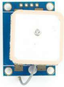
Fig. 3.5: Neo 6 GPS Receiver
