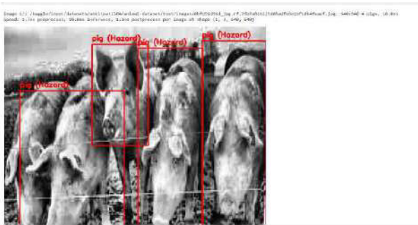
Figure 1: Hazardous Animal Detection using YOLO (Pig – Red Bounding Box)
