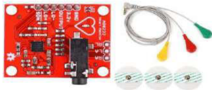
Fig. 3: AD8232 Single Lead Heart Rate Monitor
