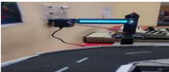
Fig 5: Display showing clear road when no vehicle is detected
