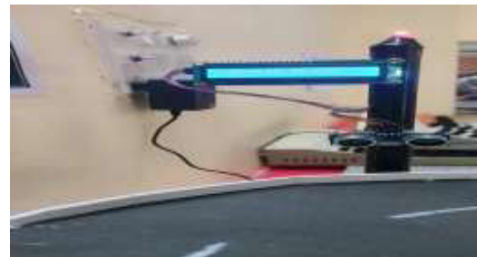
Fig 7: Display showing Vehicle Ahead Caution when sensor detects the vehicle
