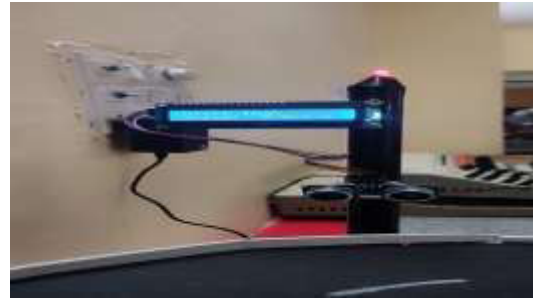
Fig 6: Display showing speed and distance of vehicle detected
