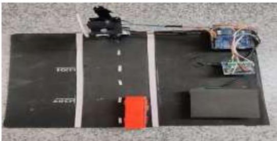
Fig 3: Model of automatic speed control system
