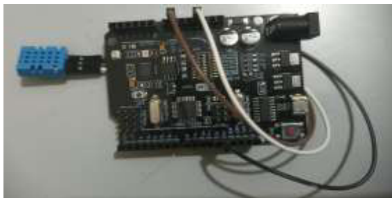
Fig3: ESP32 and DHT Sensor Interfacing Circuit.
