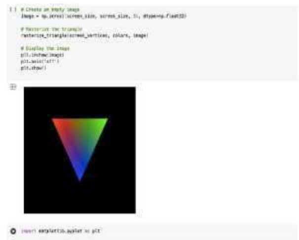
Fig 6.3.1 Expected Output of Colour shading of triangle When viewed in Google colabnotebook
