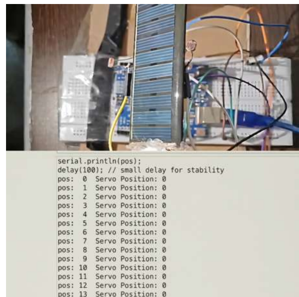
Fig. 2. Automatic Solar Tracker Output Position in 0-Degrees
