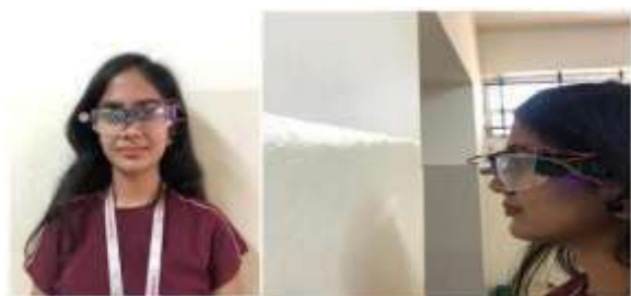
FIG 7.2: Person Wearing Smart Glasses Young woman named Sarah is navigating her home environment while wearing a pair of custom-built smart glasses. These glasses house a compact electronic system integrated into the frame: an ESP32 microcontroller acts as the central brain, powered by a small battery pack discreetly attached to the side, and a miniature ultrasonic sensor is mounted near the bridge of her nose, pointing forward. As Sarah walks confidently toward a hallway, the ultrasonic sensor continuously pings the environment with sound waves. The ESP32 rapidly processes the time it takes for the echo to return, calculating the distance in real-time. Suddenly, a subtle, but clear, beeping sound emanates from a small buzzer integrated into the earpiece of the glasses. This audible alert is triggered because the sensor has detected that she is approximately 0.167 meters (about 6.5 inches) from a nearby wall—exactly half of the preset threshold of 0.334 meters (approximately 13 inches).
