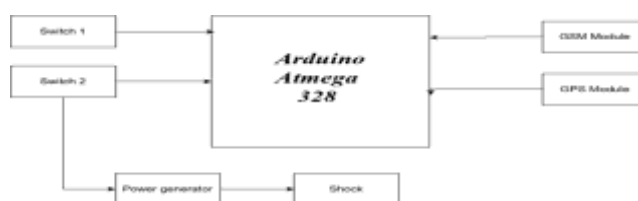
Fig. 1. Block Diagram of Self Defence Stun Gun System
